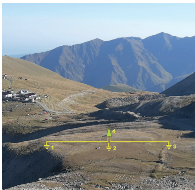
1 and 3 –ground electrodes used to measure telluric current variation, spaced 120 m from each other; 2 –ground electrode; 4 –measuring equipment point [43,03692°N76,94230° E]
